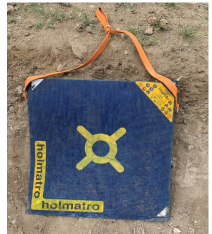
Rubberized air bag. Size: approximately 0.6 metre by 0.6 metres.
